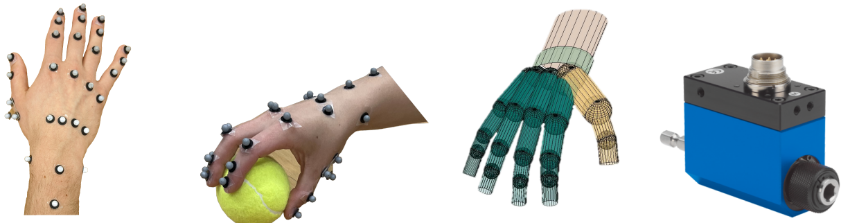
Figure 1: Hand with reflective markers for motion capturing (far left), hand during ball grasping (left), dynamic hand model (right), and torque sensor for new measurement setup (far right).
